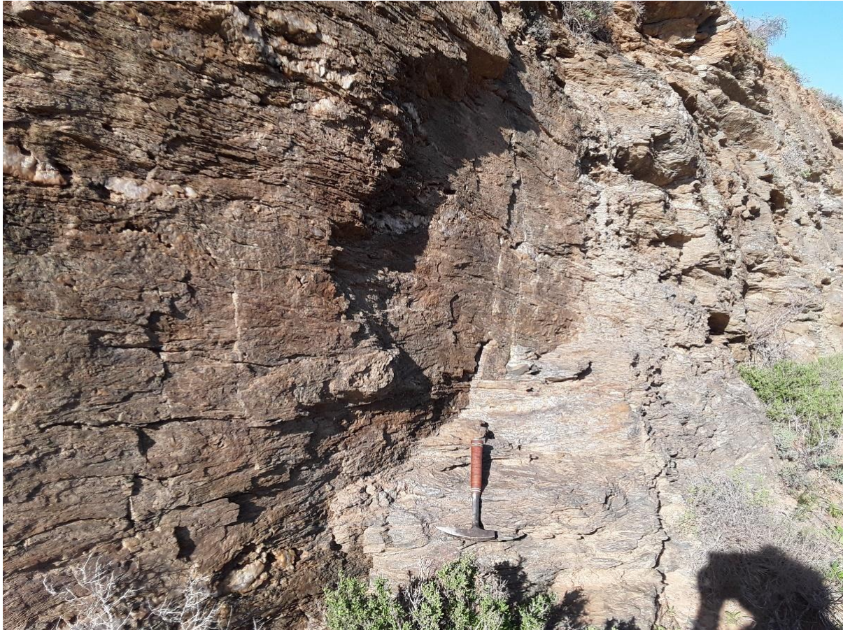
Figure 12: Schist bedrock as encountered in Zone 13, exposed in a redundant road cut
