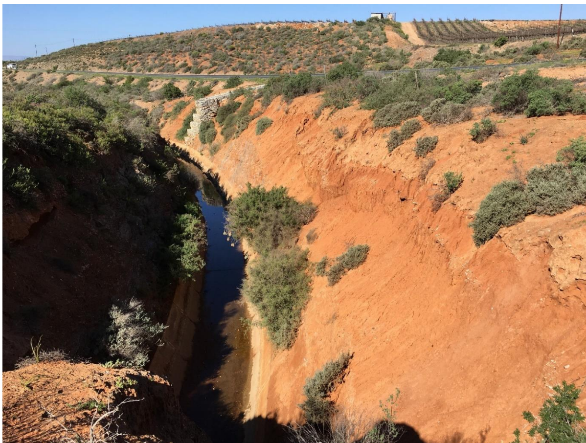
Figure 9: Zone 4 - localised deep aeolian sand profiles that can be expected across the scheme
